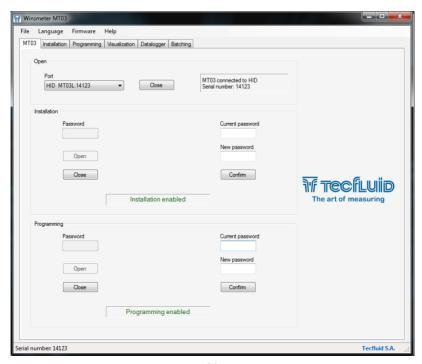
Once the password is written, press "Enter" or "Open", and the installation or programming tab will open. At the bottom of each section the text "Installation tab open" or "Programming tab open" will be displayed
