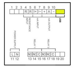
Connect the USB cable at one end to the converter and at the other to the computer where the software is installed.
