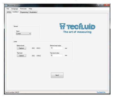
In the installation window the parameters that adapts the converter to a sensor can be configured.
