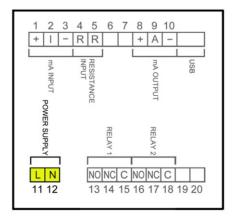
Before starting the wiring of the instrument, check that the supply voltage available is the same as marked on the label of the converter.
