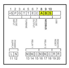
For the electrical installation it is recommended to use multiple conductor cables with individual cable sections in the order of 0.25 to 0.5 mm<sup>2</sup> in order to make it easier to connect. It is better to maintain a single cable for the MODBUS connection.
